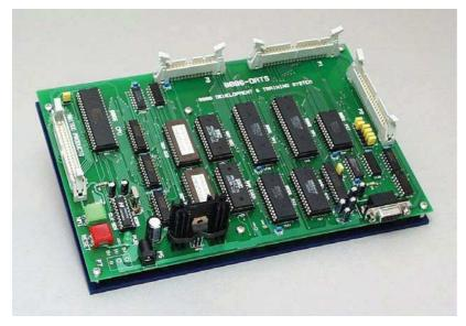
The 24-131 DATS includes a comprehensive target board based on the true 16-bit 8086 microprocessor. Designed as a general purpose unit it simplifies the teaching of the 8086 CPU & its commonly used peripherals. Suitable for use at all levels, from simple programs flashing an LED to use as a controller in complex projects. The 24-131 DATS offers a wide variety of hardware and software facilities whilst retaining simplicity in operation.
